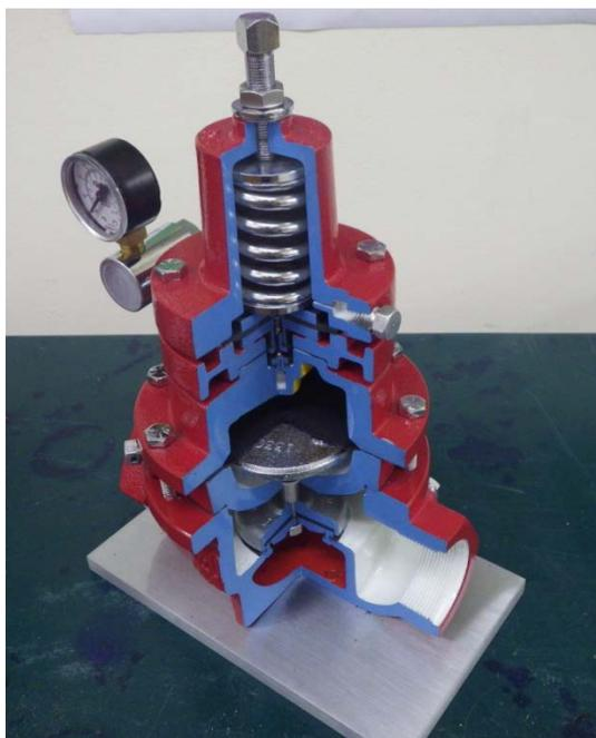
*(Left)* Gas Back Pressure Valve (AAA). This valve is typically used to regulate flow using the gas in the line – it regulates the “upstream pressure” in a system.
