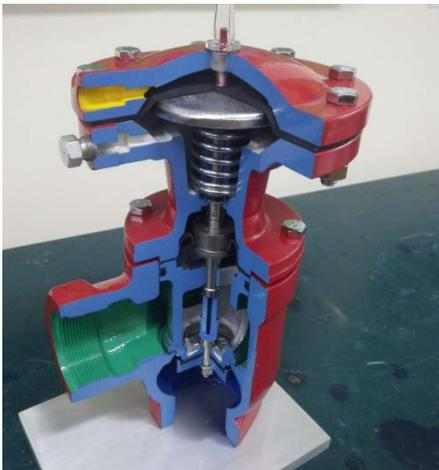
(Left) Low pressure valve Control Valve Motor Valve (EJA). Designed for liquid systems up to 500 psig.
