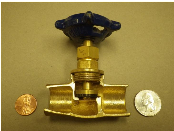
*(Left)* Cut Away view of a 1/2" water valve for a brazed or solder connection to copper pipe with handle (black). To turn this on fully requires multiple turns of the handle. U.S. 1 cent and 25 cent pieces are present for size comparisons.
