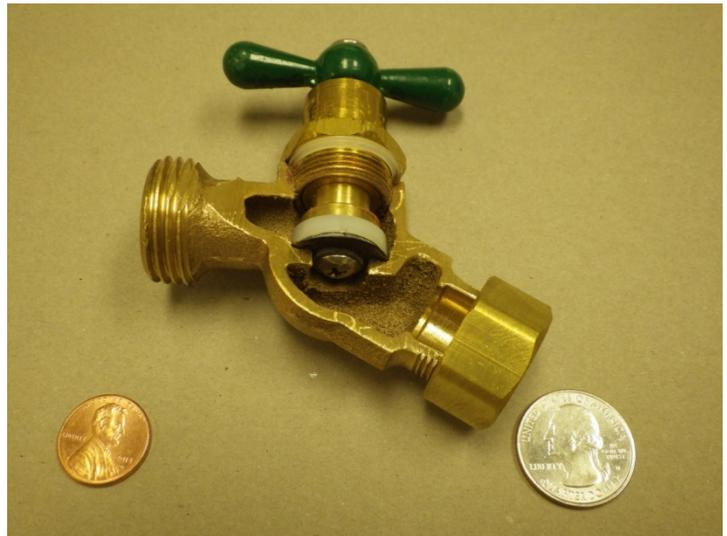
*(Right)* Cut Away view of a 1/2" water faucet valve with handle (green). To turn this on fully requires multiple turns of the handle. U.S. 1 cent and 25 cent pieces are present for size comparisons.
