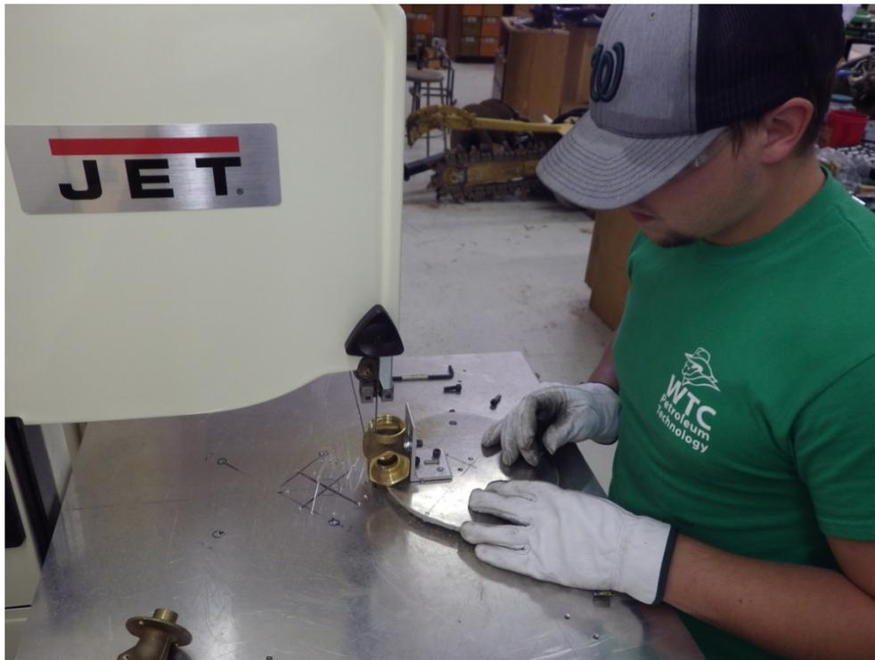
(Above) Valve being cut open to produce a cut away valve. The operation is being carried out on a JET band saw. This valve is a 1.5" ball valve. Notice that the working parts are removed for the cutting operation.
