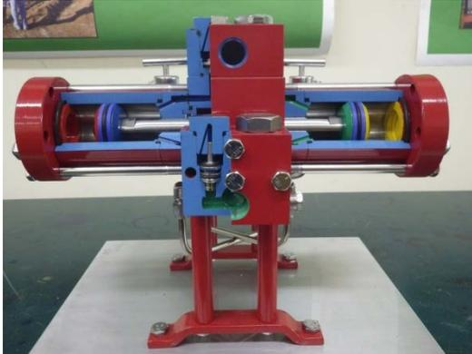
(Left) GLYCOL Pump (GAB). This item works as a pump, and is our first pump cut away unit. It pumps Glycol as the name states, which is a viscous fluid used to dehydrate (remove water) from oil, ethanol, methanol, or other petroleum products.
