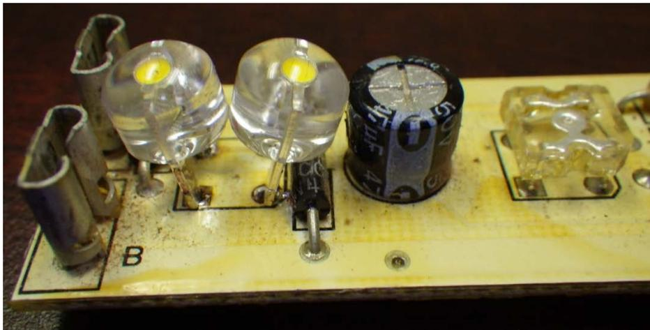
*(Above and below)* The single square LED light right side of photo was replaced by two LED lights. The Square LED lights are red. The round LED lights are white *(see below)*.
