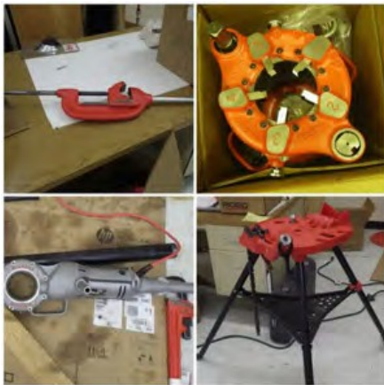
(Above) Pipe threading tools used by the students.
