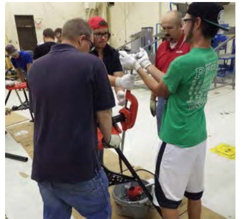
(Above) Toby Lawrence of RIDGID™ demonstrates to sophomores how to use the RIDGID™ 300 power drive pipe threading tool.
