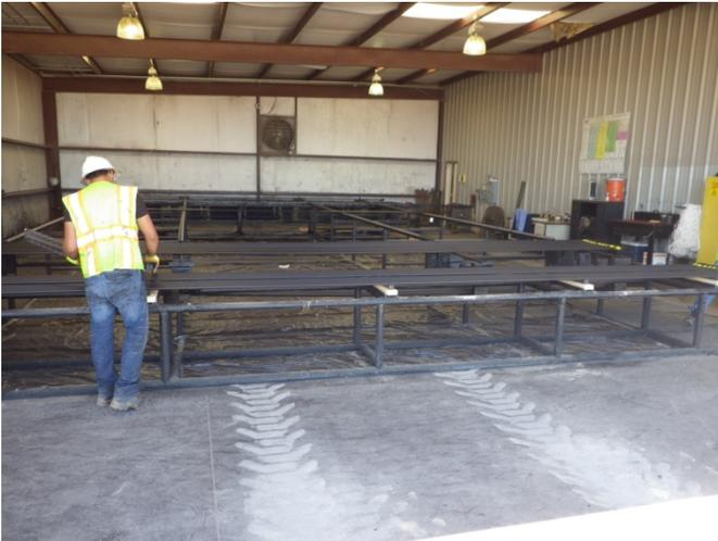
(Left) Completed reconditioned rods ready for packaging, shipping, and reuse.
