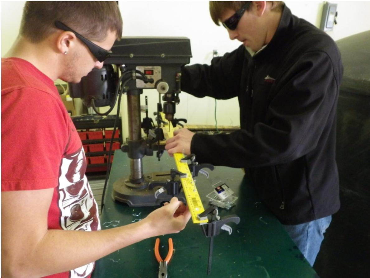
(Above) Colton Cannon and Caleb Jetter work on their project using a drill press and clamps. After drilling was completed they used a pop rivet tool to attach the two drilled rulers together.
