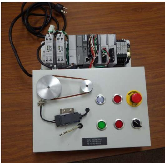
*(Left)* this is the type of unit used in the PLC training course by IDEC. Note, the two pulleys on the left hand side; these are a motor and a counter. The lights, buttons, and motor are items programmed by the PLC unit which is just above the small pulley. Remember a PLC is like a small computer.
